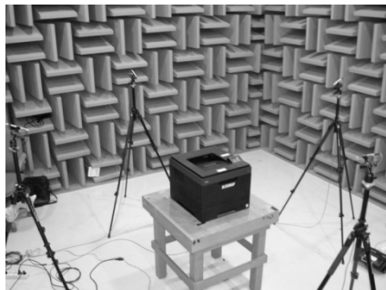
Fig. 15. Measurement of SPL of a laser beam printer in a semi-anechoic chamber.
