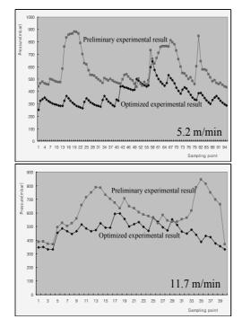
Fig. 14. Optimized results of vacuum pressure.
