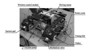
Fig. 1. Overall structure of climbing robot.
