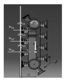
Fig. 5. Forces applied to the robot.
