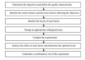
Fig. 11. The process of Taguchi methodology.
