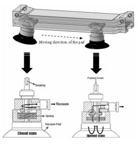
Fig. 4. Working principle of mechanical valve.
