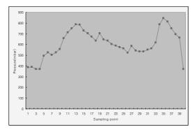
Fig. 10. Pressure change of a single suction pad (at a speed of 11.7 m/min).
