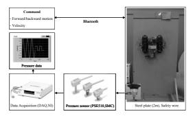
Fig. 9. Experimental setup.
