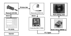
Fig. 2. Schematic of wireless control system.
