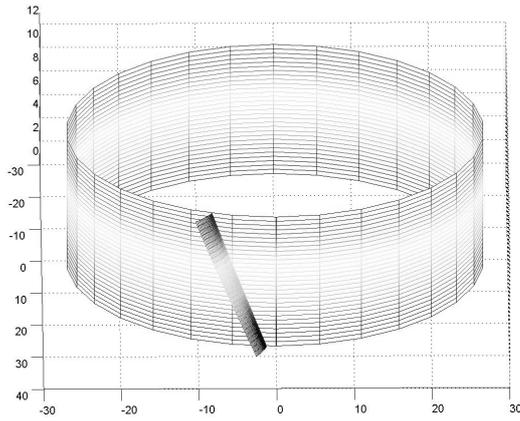
Fig. 3. Generated surface of a left-hand helical gear.
