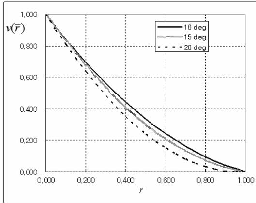
Fig. 9. Common function of deflection in the direction of circulation.
