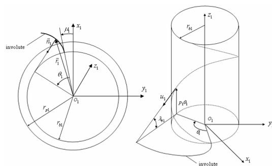
Fig. 2. Cross-section of a left-hand helical gear.
