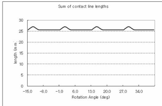
Fig. 17. Total length of contact lines.
