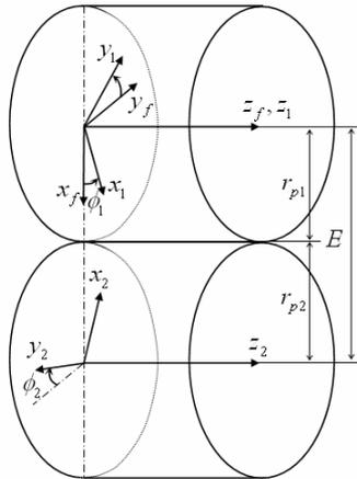
Fig. 4. Coordinate systems for a helical gear pair.
