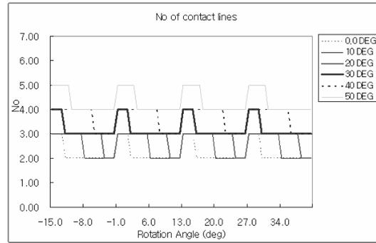
Fig. 19. Number of contact lines vs. helix angles.
