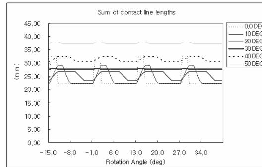
Fig. 20. Lengths of contact lines vs. helix angles.
