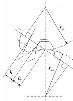
Fig. 12. Position of contact on the gears.
