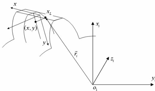
Fig. 13. Contact point projected on the gear center plane.
