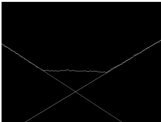
(b) Straight line extracted by Hough transform
