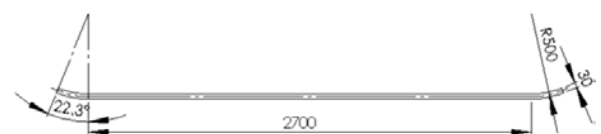
Fig. 2. Initial dimensions of the workpiece for modeling (in mm).
