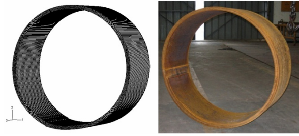
Fig. 5. Comparison of numerical and experimental results (diameter = 1000 mm).
