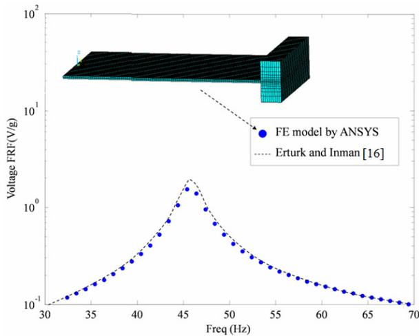
Fig. 3. FE model verification with the analytical solution.
