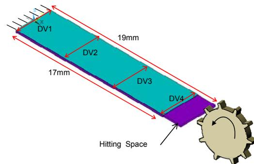
Fig. 4. Design variables in the initial model.
