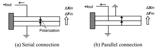
Fig. 1. Polarization of bimorph.
