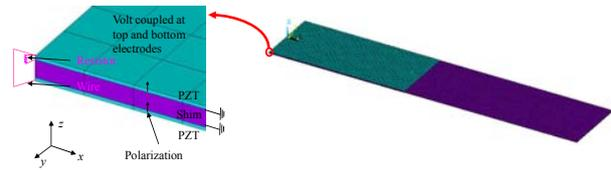
Fig. 2. FE modeling of piezoelectric bimorph using ANSYS.
