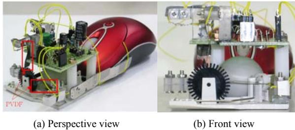
Fig. 9. Mouse with piezoelectric energy harvesters.
