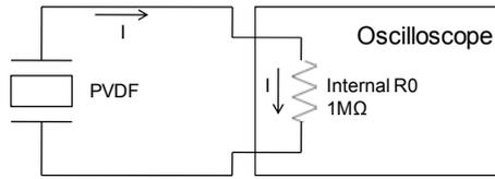
Fig. 5. Piezoelectric energy harvester with internal resistance of oscilloscope.
