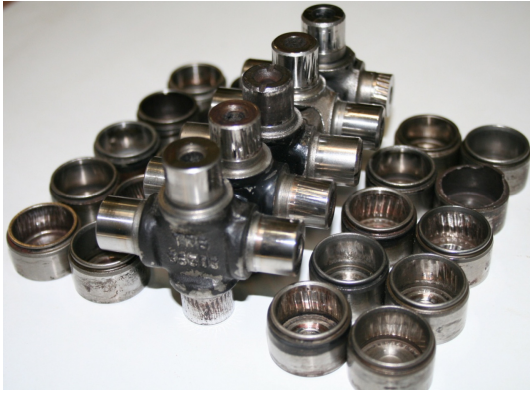
Fig. 14. Samples of the failed Cardan joints that were examined for the purposes of this research.
