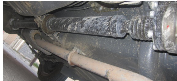
Fig. 19. Configuration of a Cardan joint with the intermediate spring and damper elements used in “ROA” automobiles.
