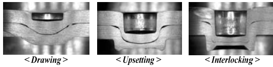
Fig. 1. Plastic deformation of the upper and lower sheet in the mechanical clinching process.
