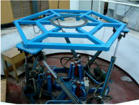
Fig. 1. Hydraulically driven 6-DOF parallel manipulator developed by the Beijing Institute of Technology.
