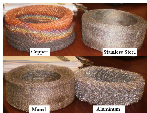
Fig. 8. Regenerator matrixes after about 15 hours of use.
